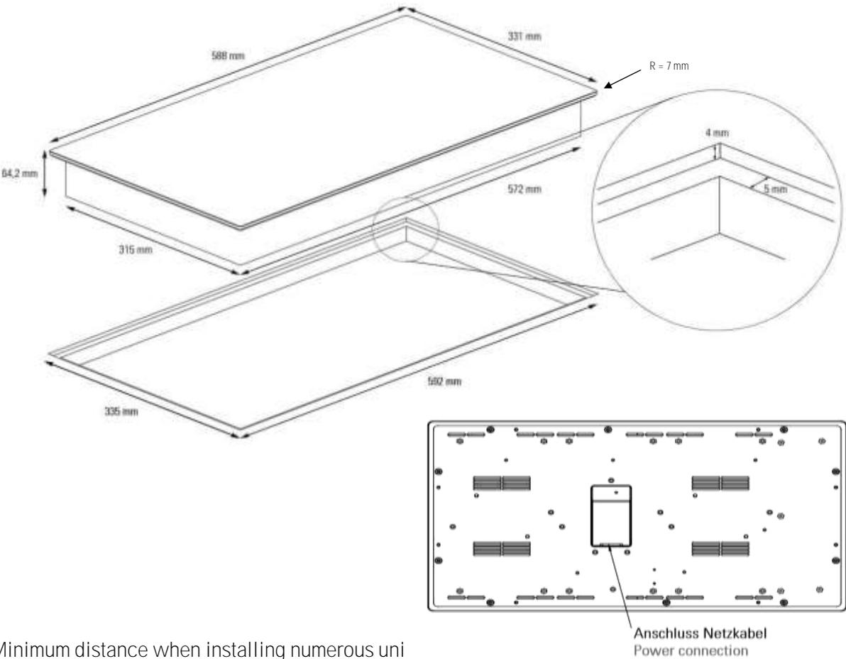
Minimum distance when installing numerous uni
