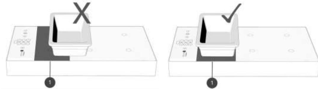
When placing dishes on top of the device or when putting them down, please take care that the edges of the dish will not scratch or damage the glass.
