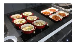
The device that is ideal for keeping food warm at the *One Dish Counter* is the induction unit InductWarm® 200 – available as table top unit or as built-in device. Each induction unit of this series comes with six induction coils, hence six pre-portioned meals can be kept warm with one unit.
