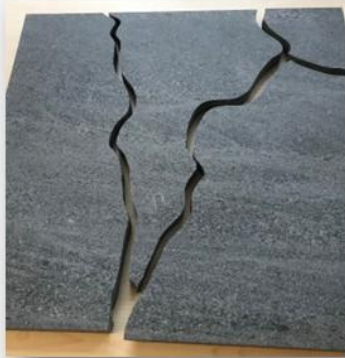
Typical Thermal Crack Curvy
